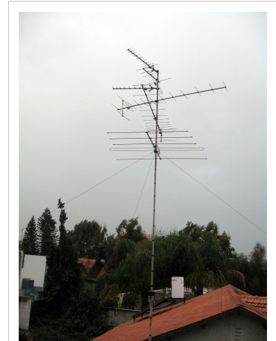
Rooftop television antennas in Israel. Yagi-Uda antennas like these six are widely used at VHF and UHF frequencies.
