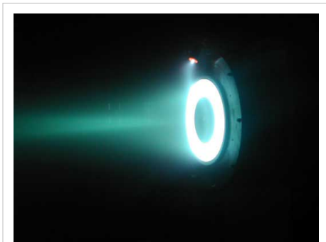
Hall effect thruster. The electric field in a plasma double layer is so effective at accelerating ions that electric fields are used in ion drives.
