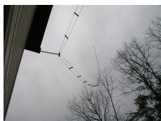
Wire dipole antenna using open-wire ladder line feedline for amateur radio use.
