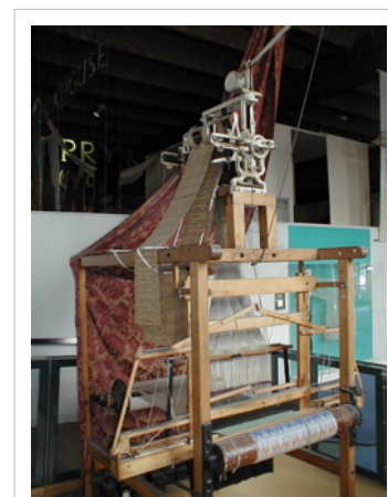
The Jacquard loom, on display at the Museum of Science and Industry in Manchester, England, was one of the first programmable devices.
