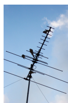
Rooftop TV antenna. It is actually three Yagi antennas. The longest elements are for the low band, while the medium and short elements are for the high and UHF band.
