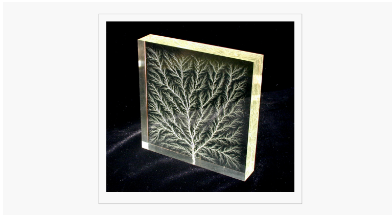
High voltage breakdown within a 4" block of acrylic creates a fractal Lichtenberg figure
